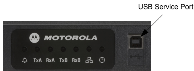
Figure 12-5 Location of USB Connector
