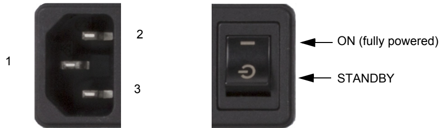
Figure 7-2 AC Power Inlet Connector and Repeater Power Switch
